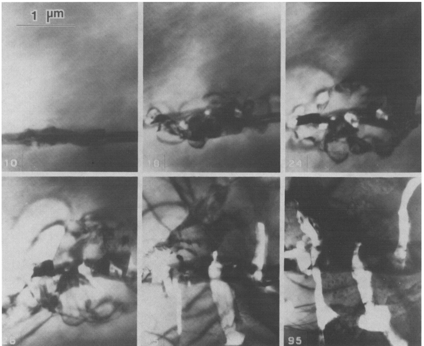
Fig. 19— A crack provides the reaction site for reduction under low reducing potential. The magnetite specimen was reduced at 514 °C using 6.6 kP 10 pct H 2 /90 pct Ar. The numbers inserted are the reducing time in minutes.
