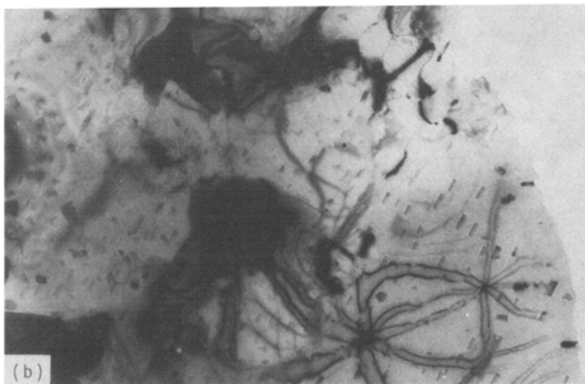
Fig. 21—(a) Rectangular magnetite nuclei occurred after heating the wustite in vacuum at 500 °C for 40 min. (b) The magnetite nuclei grew preferentially in one direction. The electron micrograph was taken after 56 min. (c) The magnetite nuclei were dissolving back into the matrix after the temperature was brought up to 600 °C for 36 min.
