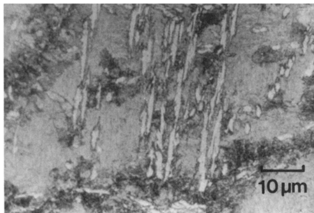
Fig. 2—Optical micrograph showing termination of the upper bainite reaction and onset of the pearlite reaction during isothermal transformation at 452°C for 32 h.
