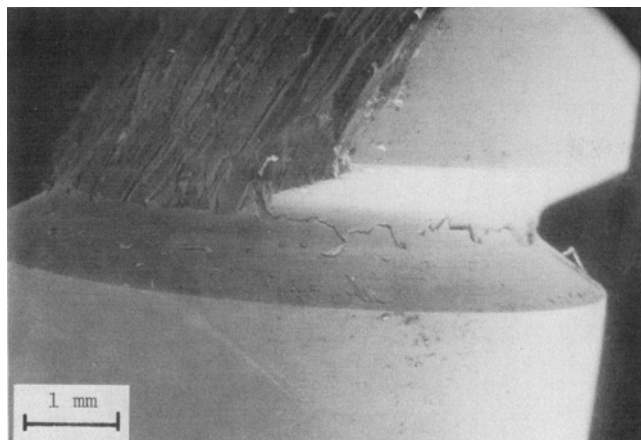
Fig. 7—Multiple initiation in the notched area of a specimen which failed by the slant fracture mode.
