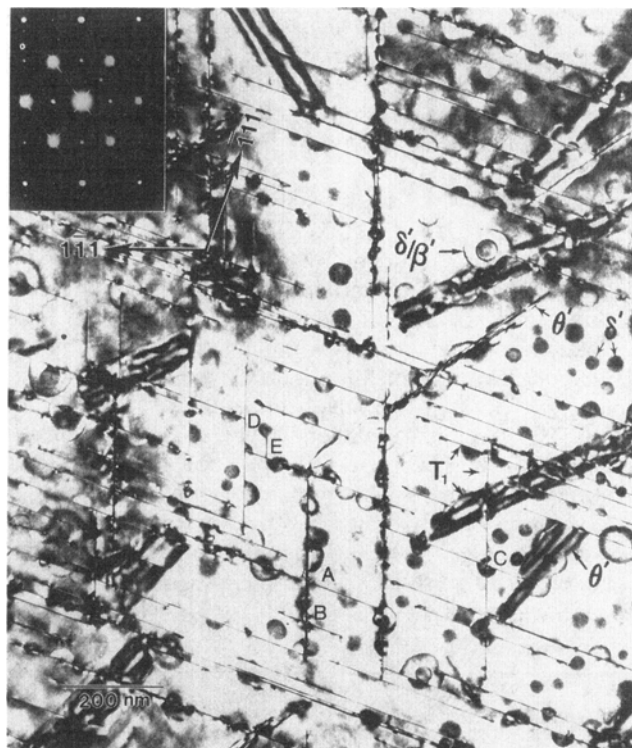
Fig. 1— \mathbf{B} = [110] orientation for material aged 72 h at 190 °C showing various phases in the microstructure. T_1 variants on (\bar{1}11) , (1\bar{1}1) , and (11\bar{1}) are marked. Inset: SAD pattern, \mathbf{B} = [110] , indicating the presence of T_1 plates on three (111) variants. \mathbf{B} = [\bar{1}2\bar{1}3]_{T_1} .
