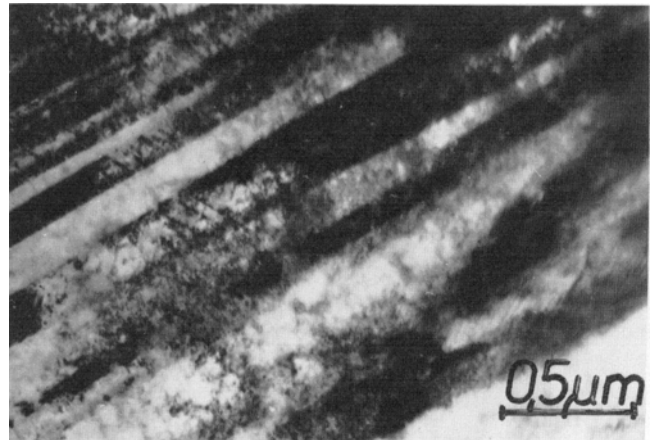
Fig. 4—Transmission electron micrograph of the martensite structure (deformation 20 pct/275°C → water).
