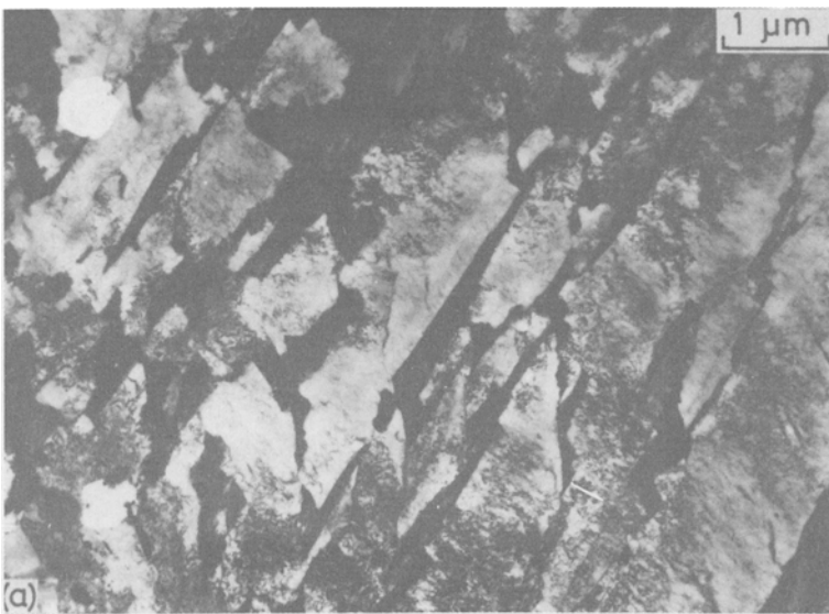
Fig. 3—Bainite laths consisting of small subunits formed by the isothermal transformation at 500 °C for 120 s of 0.20C-0.30Si-0.97Mn-1.37Cr-0.59Mo-0.0010B steel: (a) bright-field image and (b) selected area electron diffraction pattern.
