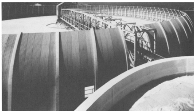
Fig. 14—Settling tank for separating magnesium hydroxide by precipitation. (Courtesy of Steetley Company).
