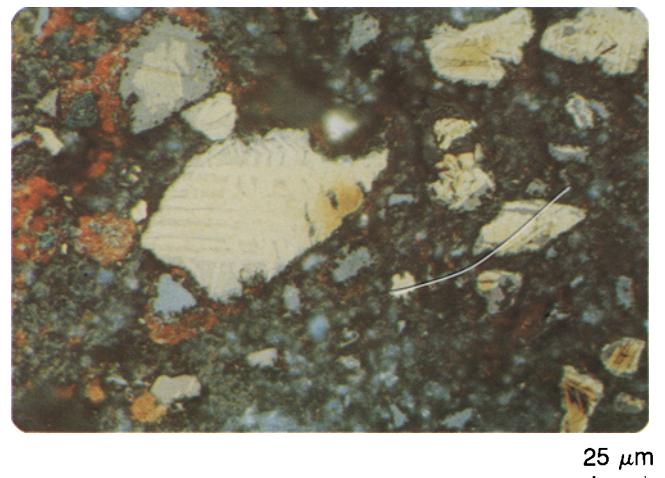
Fig. 16—Micrograph of a copper sulfide particle at the interface of a pellet oxidized at 773 K. The bright yellow phase is copper rich and recedes as the reaction progresses. The oxidation products are distinguishable by the reddish tone.
