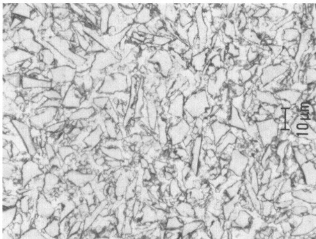
Fig. 6 - Typical microstructure of B_4C particulate specimen infiltrated with pure Al at 800 °C.
