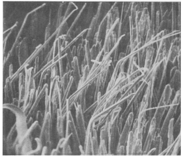
Fig. 7—Scanning electron micrograph of titanium whiskers. Magnification 200 times.
