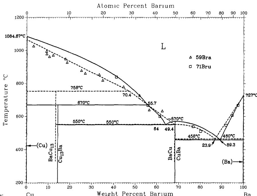
Fig. 1 Cu-Ba phase diagram.
