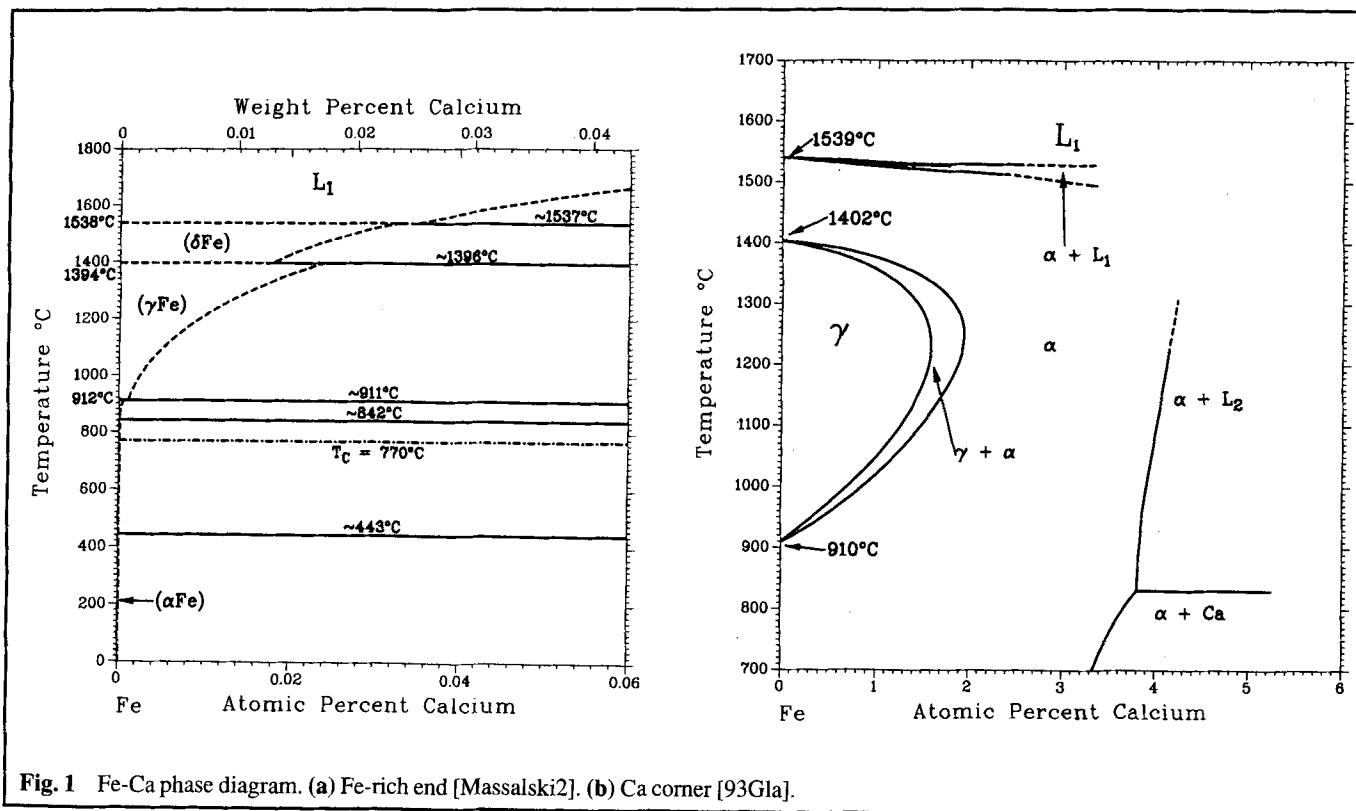
Fig. 1 Fe-Ca phase diagram. (a) Fe-rich end [Massalski2]. (b) Ca corner [93Gla].
