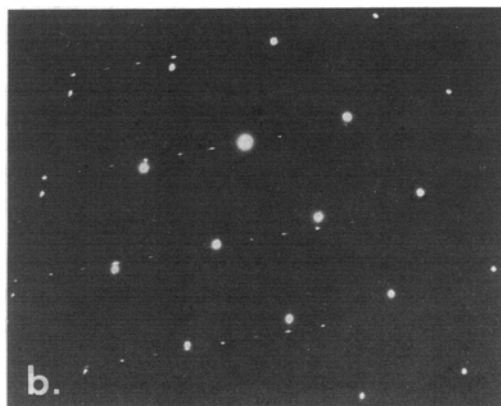
Fig. 11—(a) Transmission electron micrograph of \alpha_1 plate in Ag-45 at. pct Cd alloy aged 30 s at 240 °C; (b) corresponding SAED pattern indicating approximately parallel [\bar{1}\bar{1}1]_b and [\bar{1}\bar{1}0]_{9R} zone axes from matrix and precipitate phases, respectively; and (c) schematic indexing of (b).
