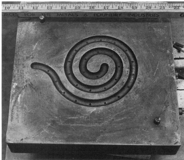
Fig. 1 Permanent spiral fluidity mold used for fluidity measurements.
