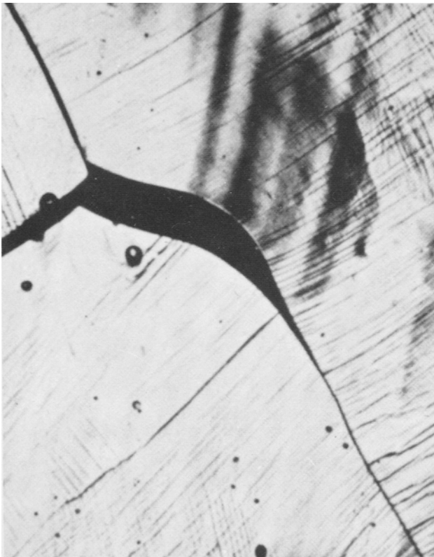
Fig. 1—A wedge crack instigated and propagated by grain boundary sliding reproduced from Ref. 5. Permission to publish granted by ASM. (Magnification for the micrograph not available).
