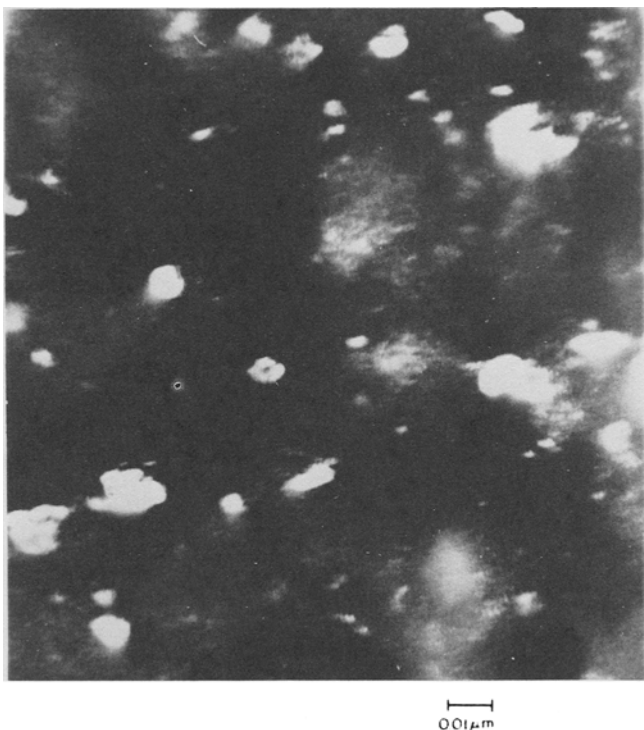
Fig. 12—Dark field electron micrograph of mechanically alloyed alloy A after vacuum hot pressing. The \text{Al}_4\text{C}_3 particles appear as white spots.
