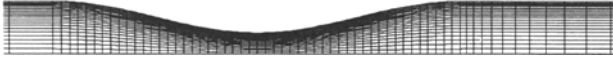
FIGURE 2. Detail of the computational mesh in the area of the stenosis. The progressive density of the mesh in the radial direction shows the carefully modelled near wall region. A progressive mesh density in the axial direction was also applied to the inlet region, so that a plug flow velocity profile that evolved into a fully turbulent velocity profile could be applied as the inlet condition.
