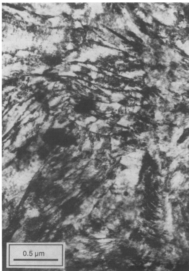
Fig. 12—TEM micrograph of the microstructure of 4340 steel at Rc 55, which consisted of undissolved alloy carbides in a matrix of heavily dislocated lath martensite.
