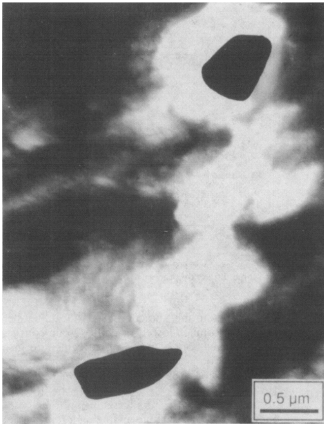
Fig. 13—TEM micrograph of microvoid nucleation around a pair of undissolved alloy carbides. The accompanying schematic illustrates the direction of shear and principal stress.
