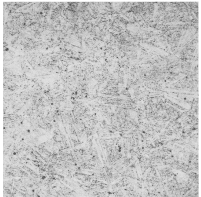
Fig. 10—Mixed martensite, austenite, and epsilon in 8 pct Cr-10 pct Mn-0.206 pct N alloy, annealed 1050 °C, and air cooled, electropolished. Magnification 100 times.
