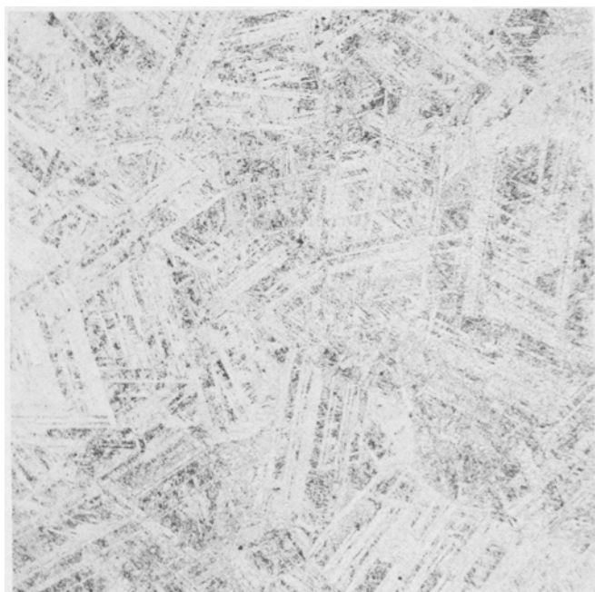
Fig. 12—Deformed austenite and martensite in 12 pct Cr-10 pct Mn-0.212 pct N alloy, annealed 1050 °C, air cooled, and cooled in liquid nitrogen, mechanically polished. Magnification 200 times.
