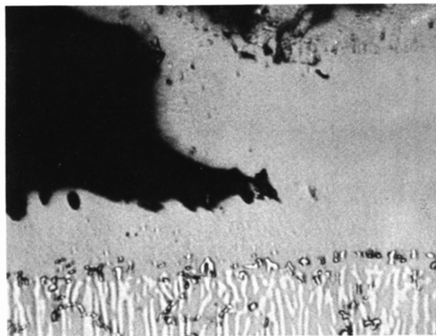
Fig. 10—Examples of delamination in coatings formed by pack aluminizing platinized IN-738; (a) Coatings formed at 0 h and (b) Coatings formed at 3 h.
