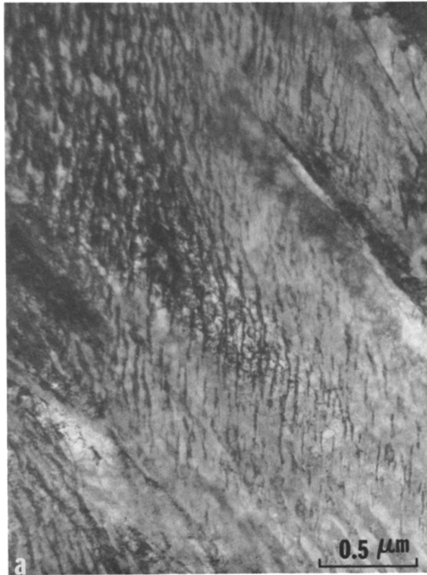
Fig. 1—(a) Structure of bainite which was obtained in isothermally transformed steel 2S54 (Fe-1.87Si-0.54C + 0.79Mn-0.3Cr) at 275°C for 17 h; (b) the corresponding selected area diffraction pattern showing a [0001]_{\epsilon} zone parallel with a [011]_{\alpha} zone.
