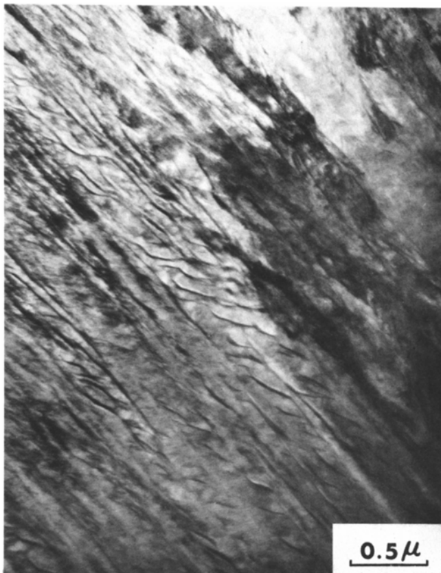
Fig. 5—Structure of bainite in steel 2S54 after isothermal transformation at 315°C for 17 min, showing unique “S-shaped” untransformed austenite and cementite.
