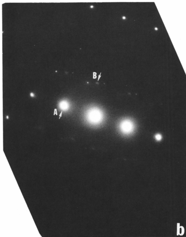
Fig. 9—Bainite in steel 2S54 obtained by isothermal transformation at 315°C for 168 h; (a) bright field micrograph showing ferrite lath with cementite; (b) the corresponding selected area diffraction pattern; (c) indexed pattern showing ferrite in [\bar{1}00] and [111] orientation and the cementite in [1\bar{2}\bar{2}] zone, no austenite is detected; (d) dark field illumination of a (201) cementite reflection showing carbides in bright contrast.
