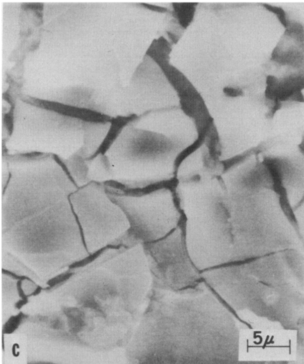
Fig. 10—Scanning electron micrograph showing a residual deposit of the test solution. (a) and (b) deposits on the actual fracture surface, and (c) and (d) deposits evaporated on a nickel plate for comparison.
