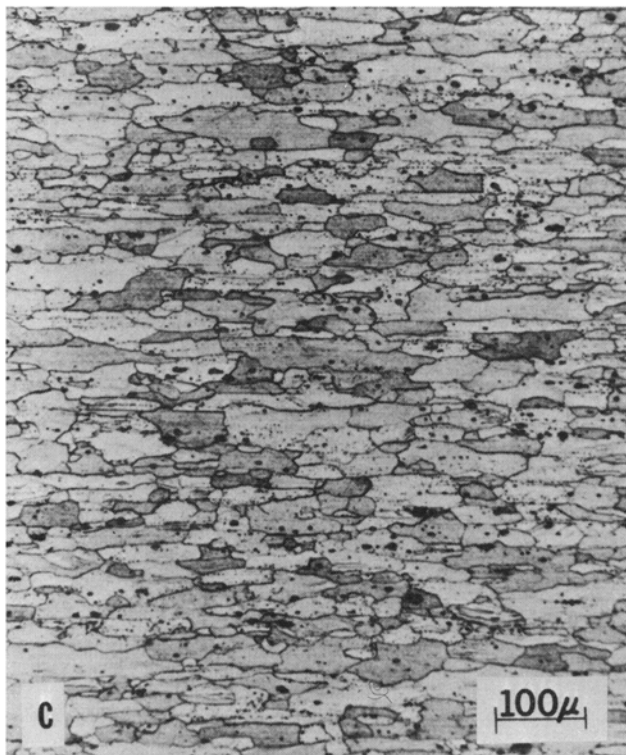
Fig. 2—Typical microstructures of 7075 aluminum sheet. (a) and (b) as received material, (c) and (d) after cold rolling from 0.080 to 0.060 in. thickness, solution heat treating and quenching. a, b viewed from the top; b, d edge view perpendicular to the rolling direction.
