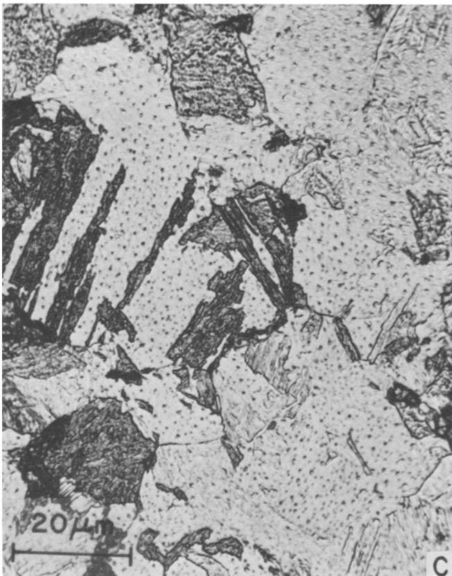
Fig. 1—Fe-3Ni-3Mo alloy isothermally annealed at 650°C: (a) 0 h—fully martensite; (b) 2 h; (c) 4 h—partially transformed; and (d) 16 h—fully ferritic.
