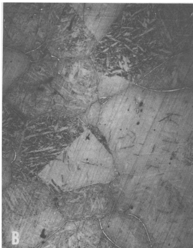
Fig. 4—Optical micrographs of proeutectoid cementite that was produced in Fe-1.43C (a) and Fe-1.49C-4.90Cu (b), by transformation at 800 °C, for one min.
