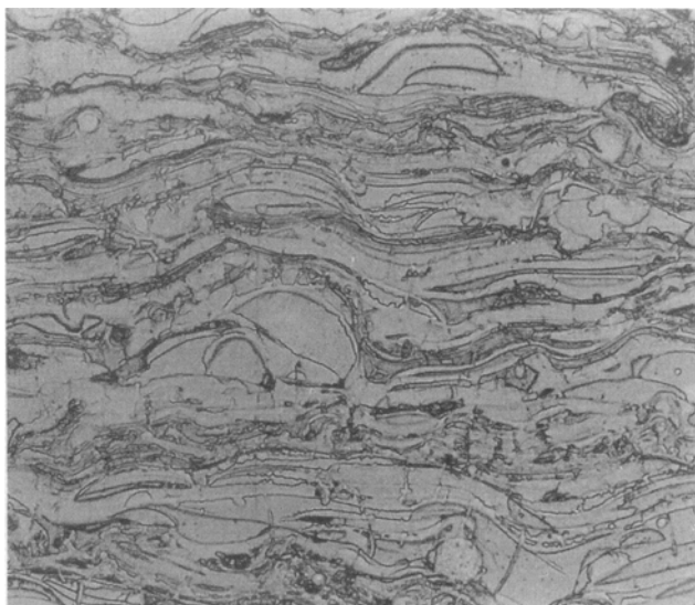
Fig. 7 Spheroidized HA coating sprayed at lower helium auxiliary gas flow rate (338 \times )
