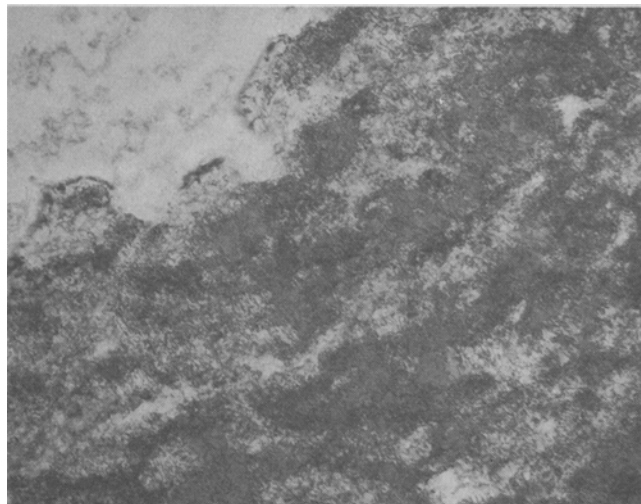
Fig. 8—Transmission electron micrograph of 2 mm-thick sheet of 7075 h.p. alloy (No. 7) in T-H10 pct A120°C for 24 h temper. Magnification 19,200 times.
