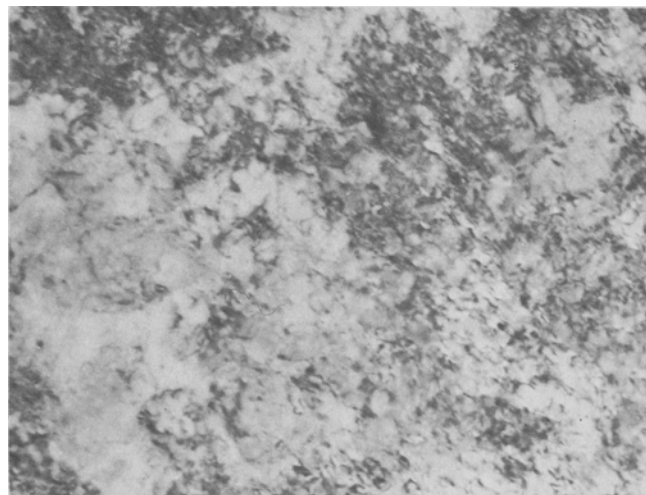
Fig. 9—Transmission electron micrograph of 2 mm-thick sheet of 7075 h.p. alloy (No. 7) in T-A105°C for 6 h H10 pct A120°C for 13 h temper. Magnification 48,000 times.
