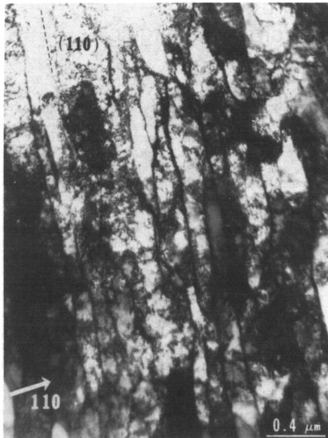
Fig. 2—Transmission electron micrograph showing the appearance of martensite laths in tempered 5.5Ni steel.
