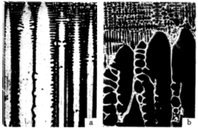
Fig. 5—Photomicrographs of longitudinal sections of Ni-14.0 at. pct Al-4.2 at. pct Cr dendritic monocrystals continuously grown at 0.25 m/h and coarsened for (a) 0 s and (b) 90 s prior to quenching the remaining liquid. Magnification 39.5 times.
