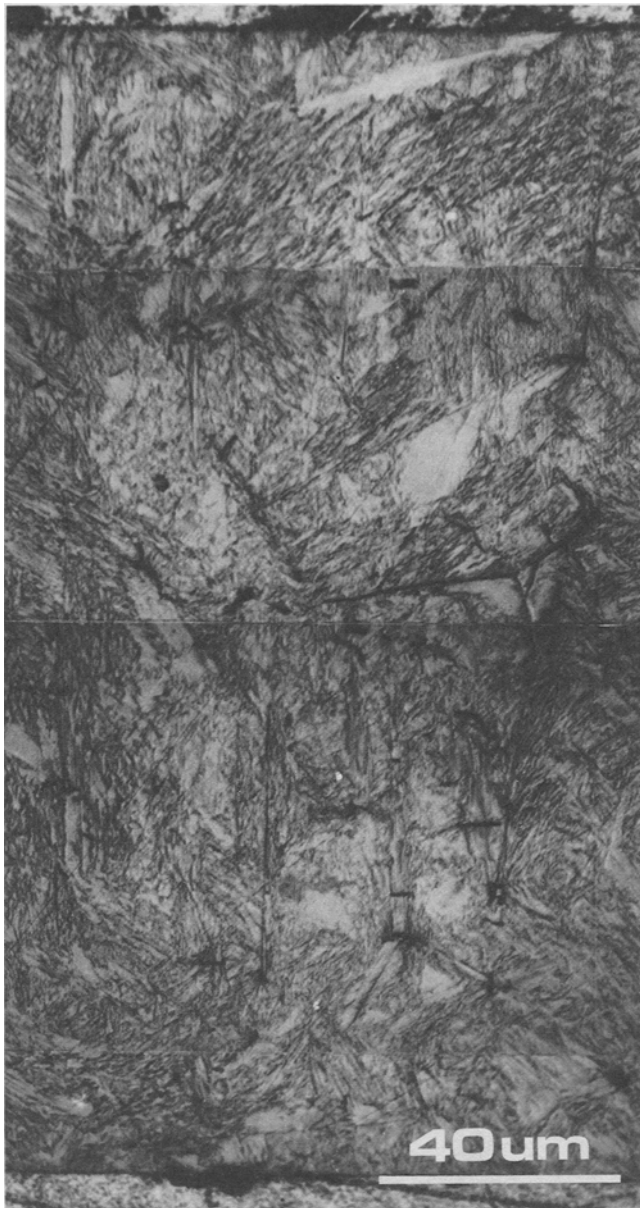
Fig. 1—Optical micrograph (composite) of cross-section of carburized specimen quenched in brine. Etching reagent: 0.5 pct Nital.
