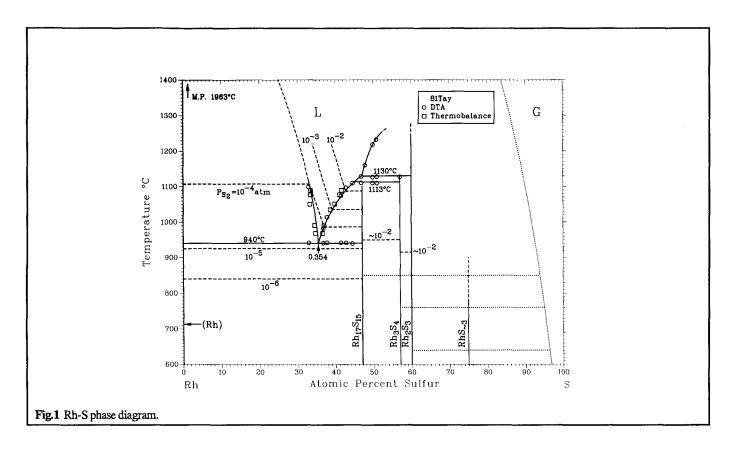
on heating. [81Tay] determined the Rh-S phase diagram (0 to 60 at.% S) by DTA and the thermobalance method under pressures sufficiently high to suppress boiling of the compounds (Fig. 1). [81Tay] observed the L  $\leftrightarrow$  (Rh) + Rh<sub>17</sub>S<sub>15</sub> eutectic point at 35.4 and 940 °C, whereas [71Zwi] observed it at 37.5 at.% S and 925 °C.
