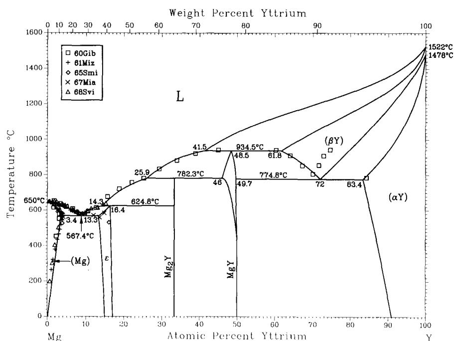
**Fig. 1** Mg-rich part of the Mg-Y system.
