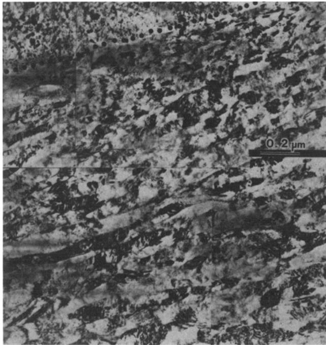
Fig. 8 Very fine lamellar boundaries immediately below the surface. The surface is marked by a dotted line.
