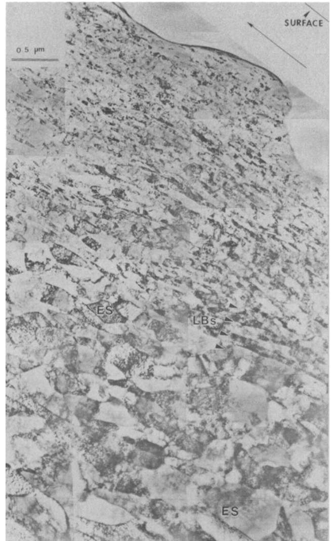
Fig. 7 The deformation structure from 0.5 to 6 \mu\text{m} below the surface is shown in this TEM micrograph of a cross-sectioned friction sample following sliding with a normal pressure of 12 MPa and at a sliding speed of 25 mm/s. The structure is composed of lamellar boundaries (LBs) nearly parallel to the sliding direction, cells, and equiaxed subgrains (ES). The microstructures at the top of the figure continue to the surface but at a slightly reduced size scale. The extremely fine long lamellas nearest the surface at the top of the figure contain both cells and deformation twins, whereas the LBs shown in the bottom of the figure contain only cells. Note the many equiaxed subgrains found at the bottom of the figure. The sliding direction is marked with an arrow. The location of the surface is indicated with a line in the top righthand corner and was extrapolated from an adjacent region in the TEM thin foil. The wavy diagonal line at the top righthand side of the photo is just the edge of the TEM thin foil.
