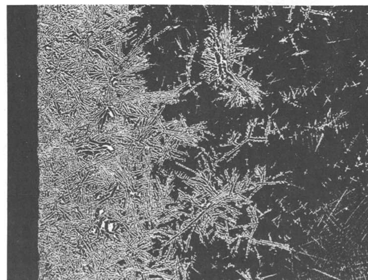
Fig. 3—Successive sections through sample shown in Fig. 2(a). (a)-(c) and traced outlines to emphasize continuity of eutectic colonies. Magnification 21 times.
