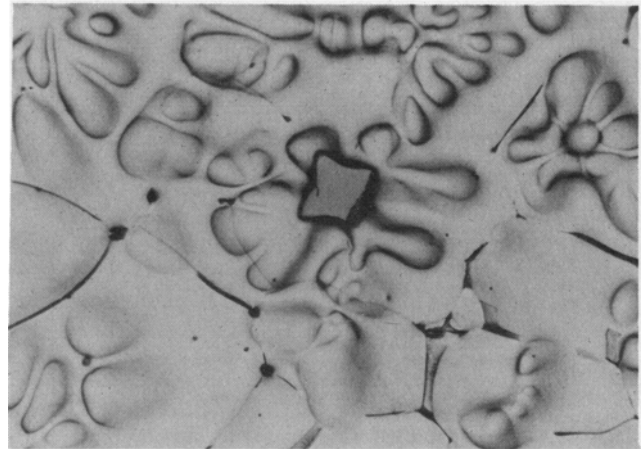
Fig. 11—Irregular intermetallic particle in Al-0.35 Ti alloy cooled at 4°C/sec. Magnification 200 times.
