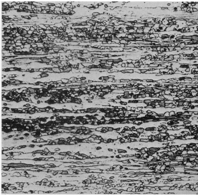
Fig. 12—Microstructure of AR ISML-ITMT 7075 plate (1 in. thick) produced following Treatment 11 in Table I and given the T6 temper. Longitudinal section. Magnification 100 times. Keller's etch.
