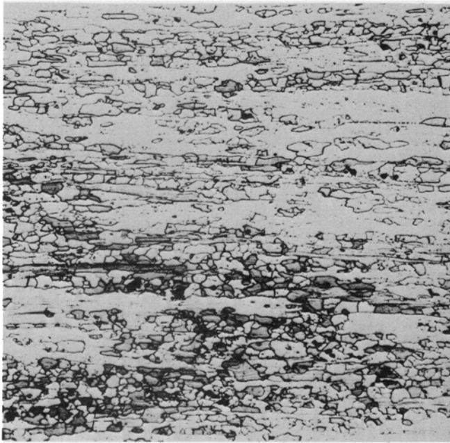
Fig. 11—Microstructure of AR ISML-ITMT 7075 plate (1 in. thick) produced following Treatment 10 in Table I and given the T6 temper. Longitudinal section. Magnification 100 times. Keller's etch.
