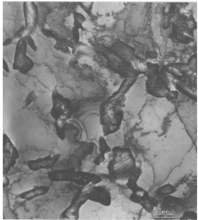
Fig. 10—Bright-field image of fine \mu -phase precipitates in alloy #3A aged at 1523 K (1250 °C)/100 h + 1123 K (850 °C)/1000 h.
