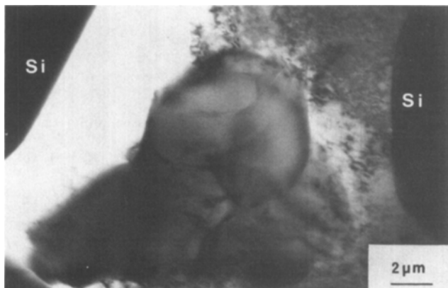
Fig. 9— \alpha (bcc) particle in the eutectic of Alloy 1 at position A after T6 heat treatment.
