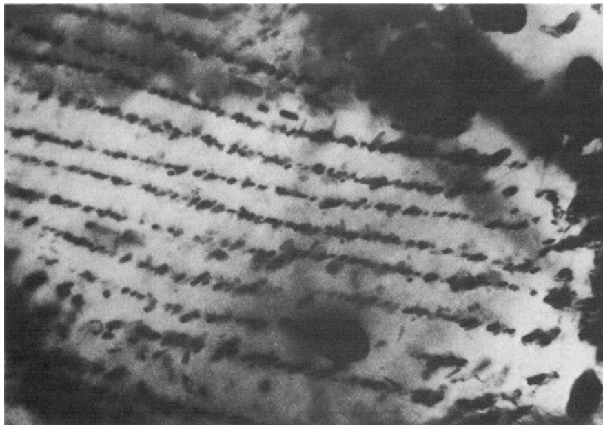
Fig. 3—Fe-1V-0.2C alloy continuously cooled \sim 10^\circ\text{C} per min; thin foil, magnification 23,000 times.
