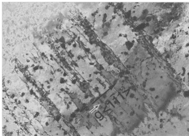
Fig. 2—Typical TEM micrograph of a replica for slip step height measurements.
