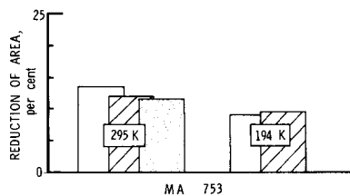
Fig. 7—Ductility of aged and annealed MA 753 at 194 K and 295 K. Key to tests as in Fig. 4.
