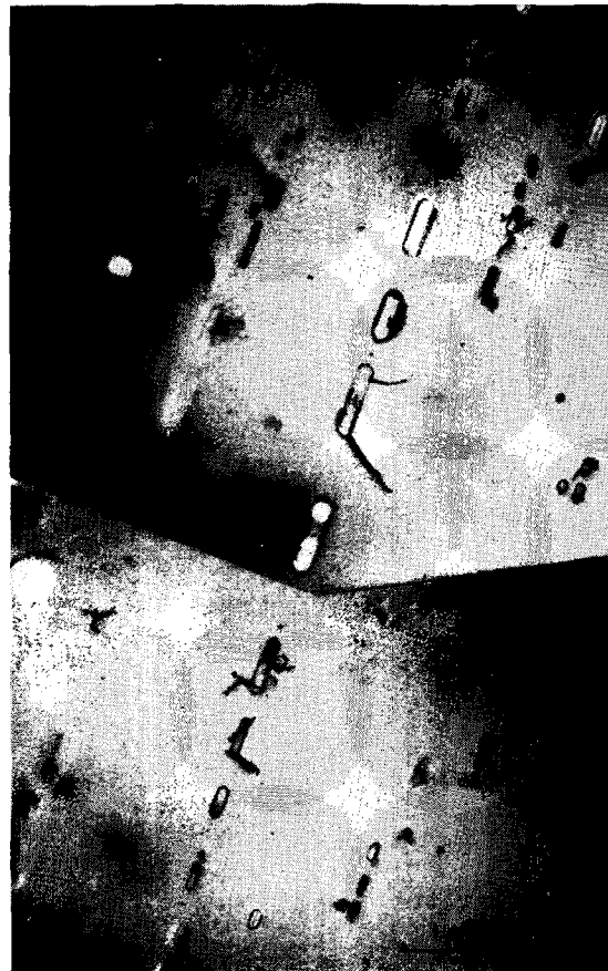
Fig. 1—Rows of bubbles containing moving liquid potassium in 2.1 mm diam. doped tungsten wire annealed at 3020°C for six min. in hydrogen. 650 KV.
