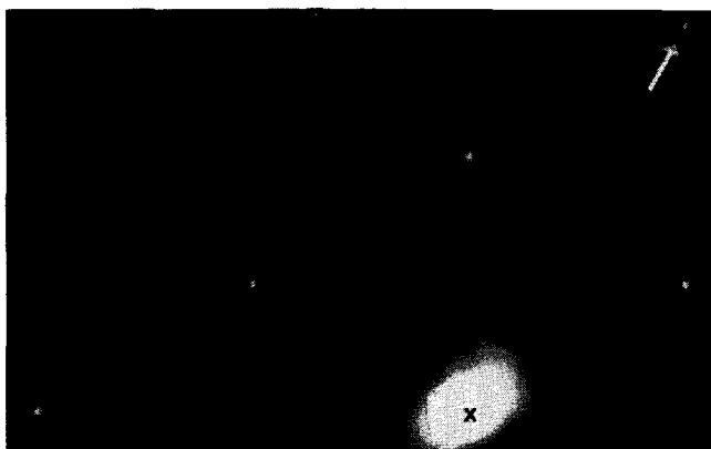
Fig. 7—Increase in matrix spot streaking in \langle 112 \rangle (example shown by arrow) with distance from the incident beam (X). Superimposed (111) diffraction patterns of tungsten and potassium from the area of a bubble similar to that shown in Fig. 5(d).
