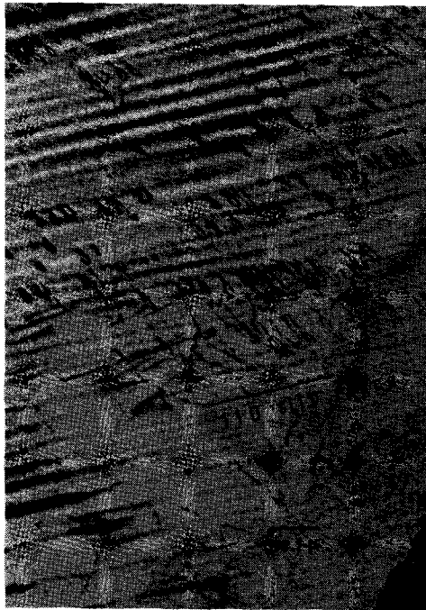
Fig. 8—Slip traces and coplanar dislocation loops in a deformed crystal. These features are similar in appearance but different in structure from “spontaneous microtwins” reported elsewhere. 4
