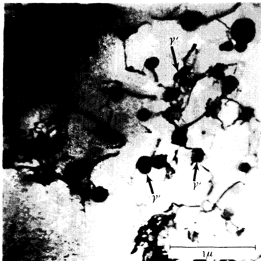
Fig. 11—Thin foil showing gamma prime phase in specimen exposed to 1400°F (760°C) and 15 ksi (103 MPa) for 10,330.5 h. Magnification about 38,000 times. Specimen No. 2.
