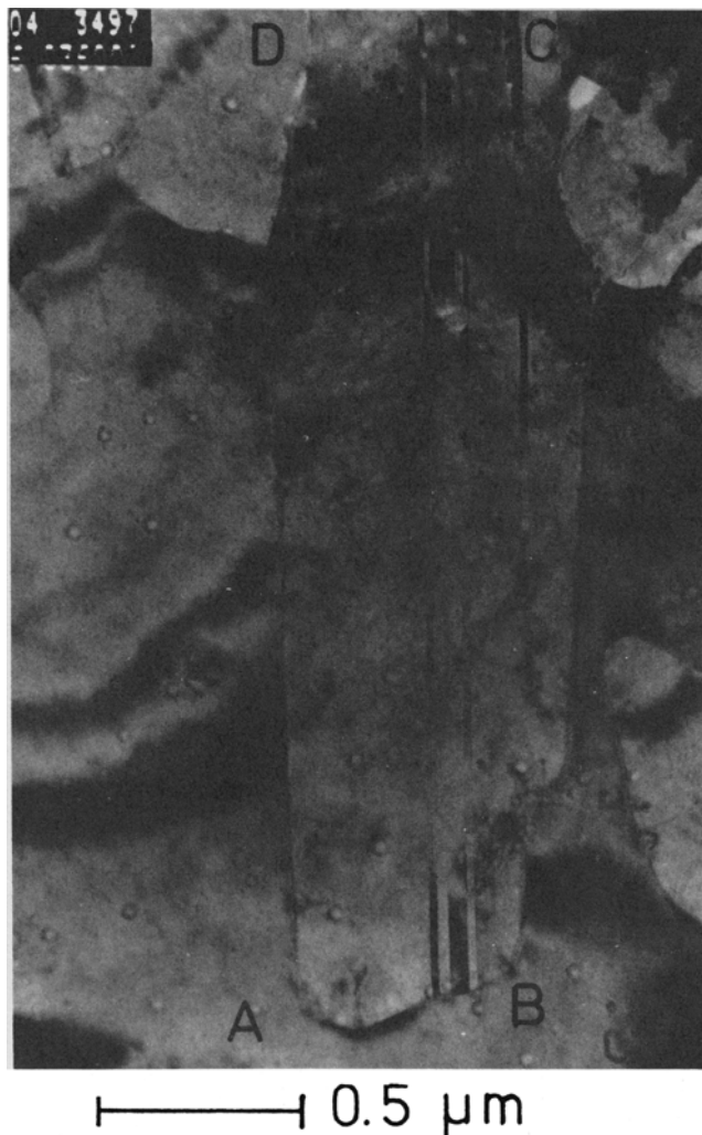
Fig. 2— \text{MgH}_2 -precipitate in Mg inside points A, B, C, D. Note internal twin boundaries which are of \{011\} type. BF, 120 kV, kinematical.
