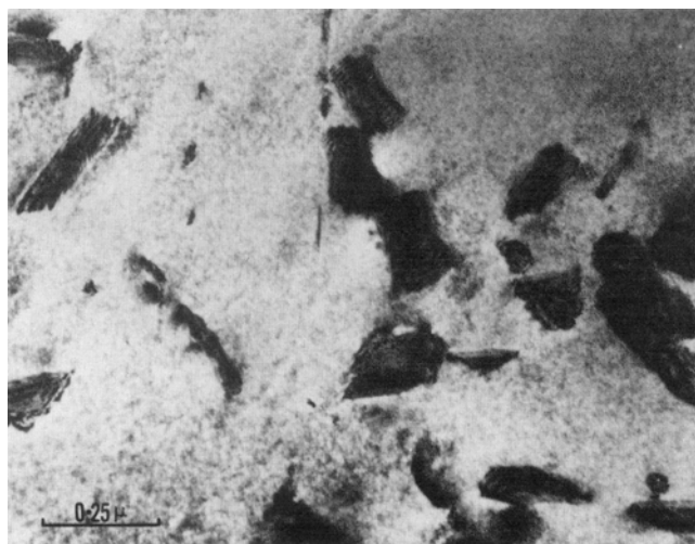
Fig. 7—Bright field electron micrographs illustrating the displacement fringes observed when the specimen was tilted from the orientation corresponding to Fig. 6.
