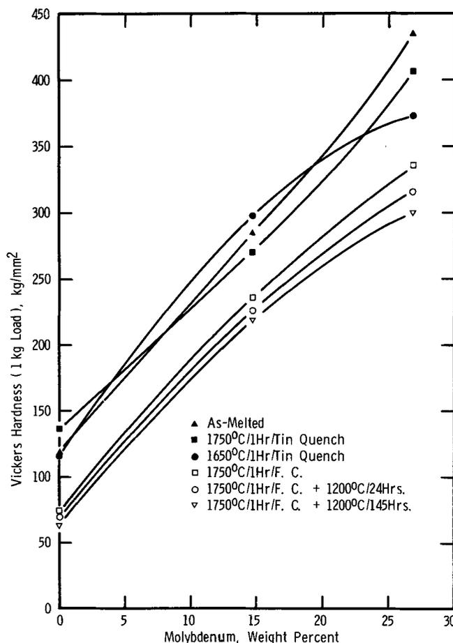
Fig. 2—Hardness of Nb-Mo-0.1C alloys vs molybdenum content in various heat treated conditions.
