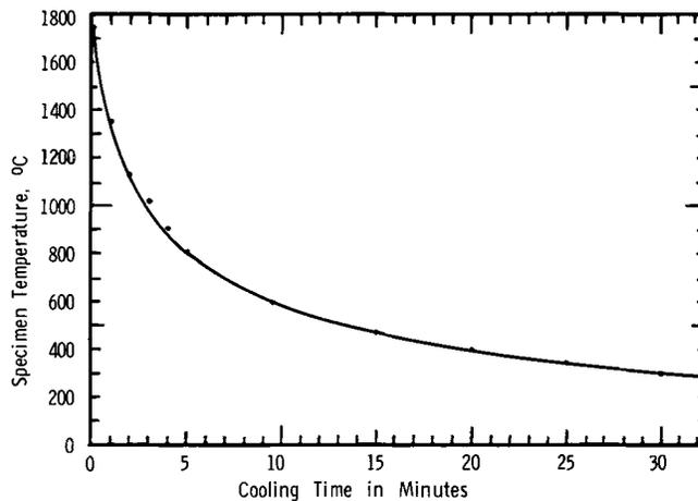
Fig. 1—Cooling curve for specimens annealed at 1750°C (furnace cooled). Total weight of specimens is approximately 30 g.
