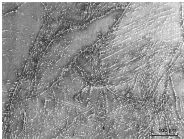
Fig. 1—Scanning electron micrograph of a sample aged at 1173 K/60 s showing grain and deformation twin boundary precipitation.
