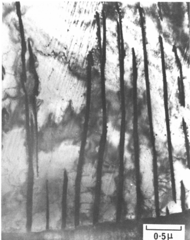
Fig. 3—An Fe-12 pct Cr-0.2 pct C alloy isothermally transformed 15 min at 750°C. Coarse laths of M_{23}C_6 . Thin foil electron micrograph, magnification 31,000 times. (Campbell).
