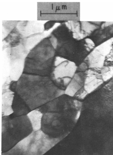
Fig. 18—Recovered structure of Fe-0.18 pct C martensite tempered 10 min at 600°C (1112°F) (electron transmission micrograph). 12
