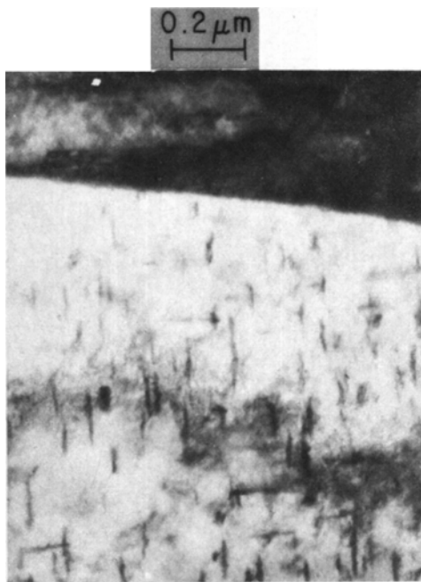
Fig. 14—Precipitation of Fe_3C during quenching in AISI 4315 steel. 7
