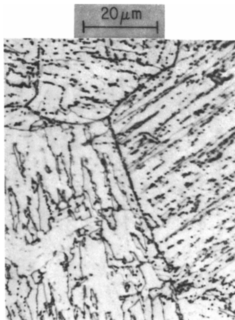
Fig. 17—Recovered structure of Fe-0.18 pct C martensite tempered 10 min at 600°C (1112°F) (light micrograph). 12
