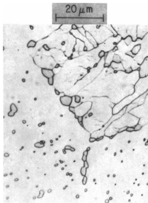
Fig. 19—Partial recrystallization in Fe-0.18 pct C martensite tempered 96 hr at 600°C (1112°F) (light micrograph). 12
