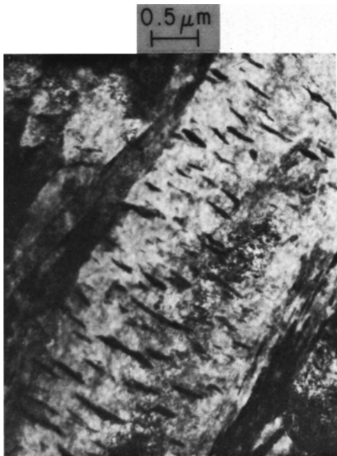
Fig. 13—Precipitation of Fe_3C in Fe-0.39 pct C martensite tempered 1 hr at 300^\circ C ( 572^\circ F ). 12
