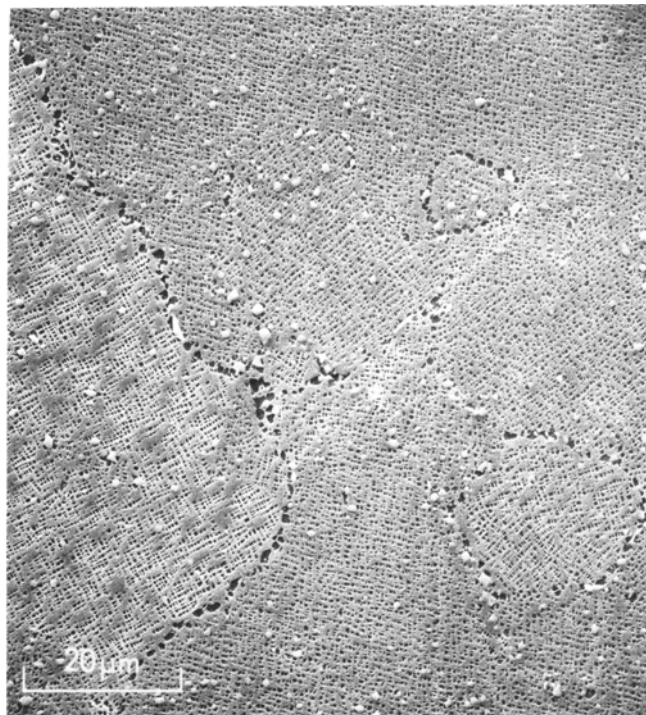
Fig. 2—SEM micrograph of the AF2-IDA microstructure showing the morphology of the grain boundary \gamma' and cooling \gamma' , as well as the carbide distribution.
