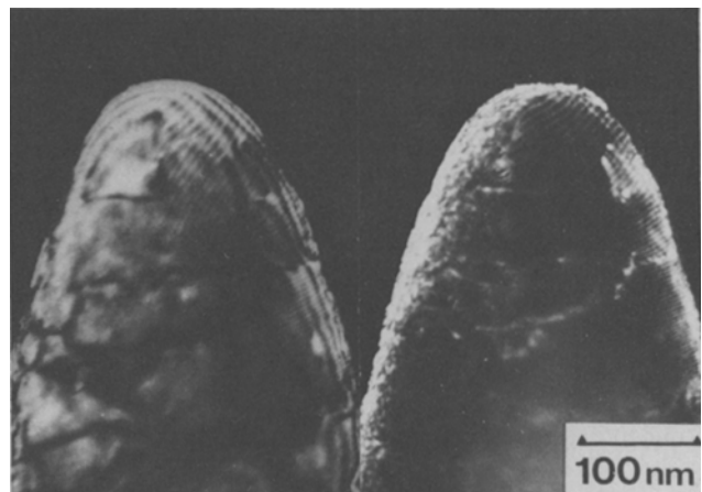
Fig. 2—Complementary transmission electron microscope images of the specimen of Fig. 1, showing periodic array of dislocations in the lath boundary. Some matrix dislocations are also visible.
